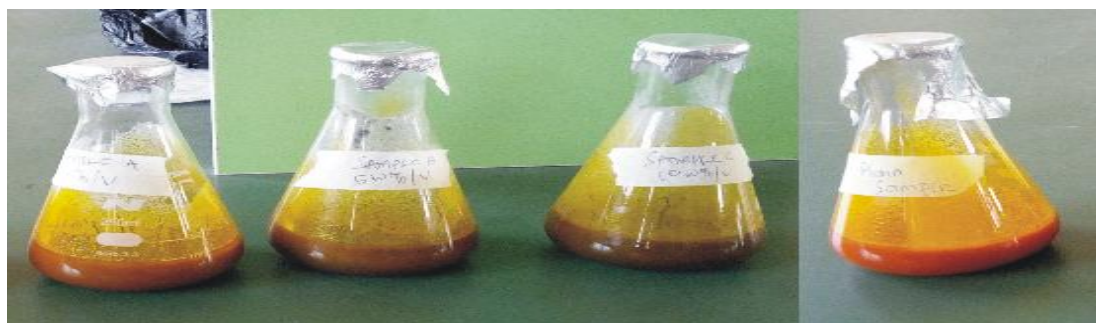
Sample A RHA 2wt%, Palm Oil (100ml) Sample B RHA 5wt%, Palm Oil (100ml) Sample C RHA 10%wt Palm Oil (100ml) Sample D Fresh Sample Palm Oil (100ml)
