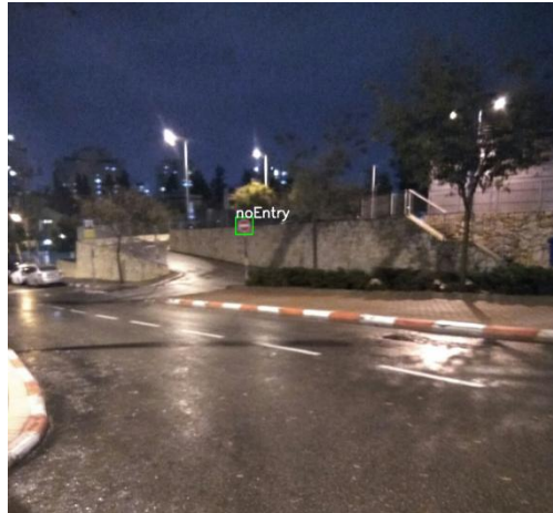
Fig. 17: No Entry traffic sign identification with tough environment conditions
