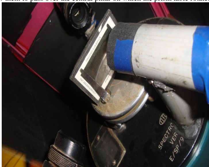
FIGURE 1.1 Photograph of detector placed in a PVC pipe on a spectrometer
