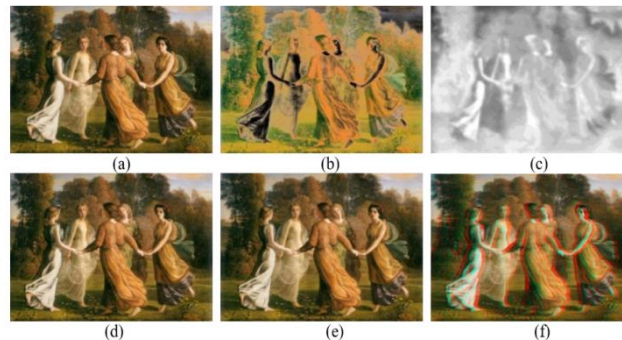
Figure 3. (a) Input Image (b) Simulated Haze Image (c) Estimated Depth Map, (d) and (e) Left-view and Right-view Images, Respectively (f) Stereoscopic Conversion Result
