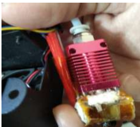
Figure 2. The damaged extruder, the nozzle head has leaked
