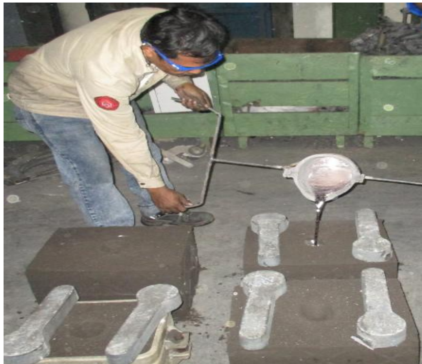
Figure 3. Pouring liquid into the mold
