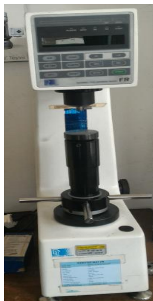
Figure 5. Rockwell FR-1e Future-Tech Corp hardness testing machine
