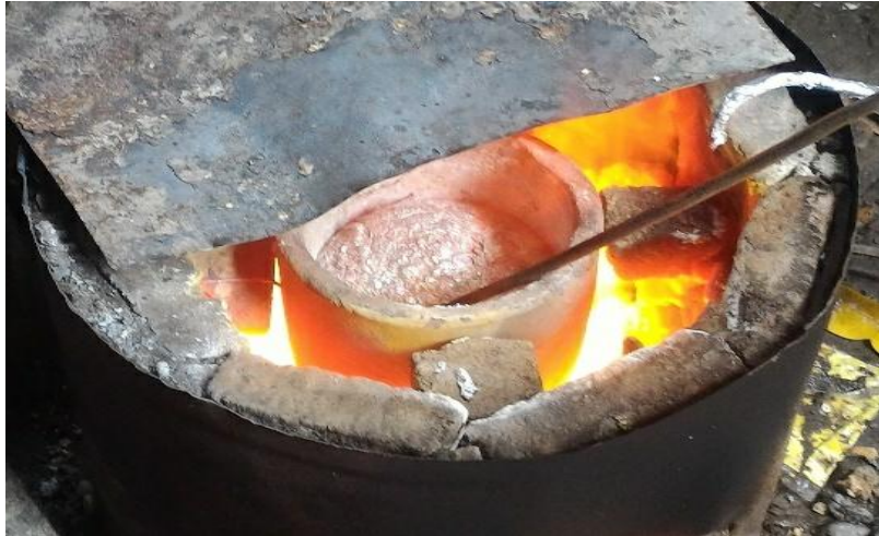
Figure 2. Degasser administration in cast fluids
