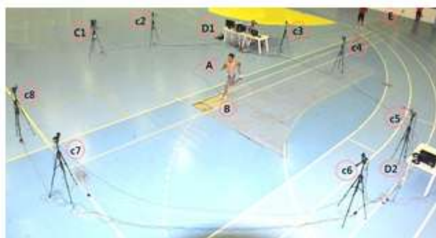
Figure 1 Experimental work (3D-Motion Capture). A: Athletic runner, B: Force platform, C (1-8): Cameras &Infrared light, D (1-2): Computer system analysis, E: Sync laser system
