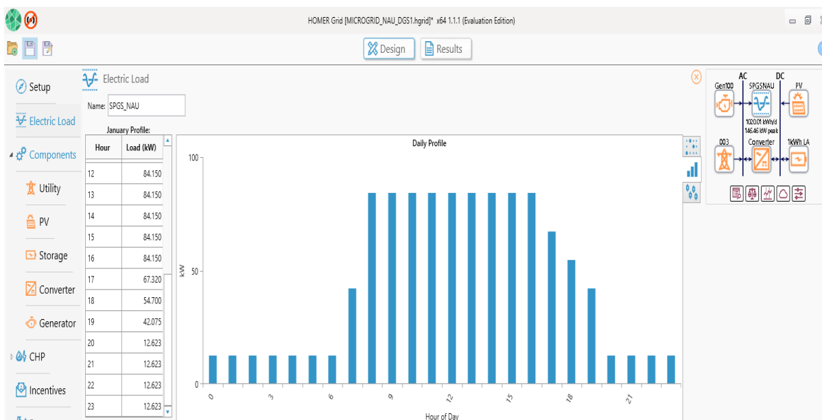
Figure 3: Load profile for SPGS Sub-grid
