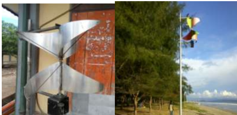
a Prototype of the Results of the Design b Installation of the Mill in the Field Fig 7. Results of Designing Windmill Hemi-Savonius Multi-Level Blade
