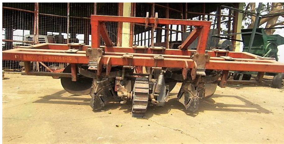
Figure 1: View of the Fabricated Two-Row Yam-Sett Planter.
