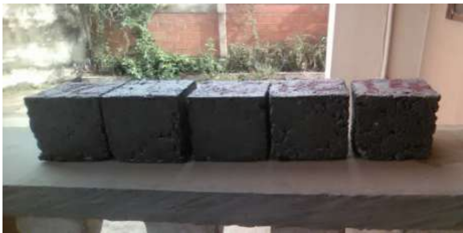
Figure 4: Concrete Cubes Before Immersion in Acid
