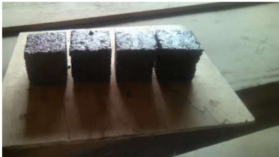
Figure 5: Concrete Cubes After Immersion in Acid
