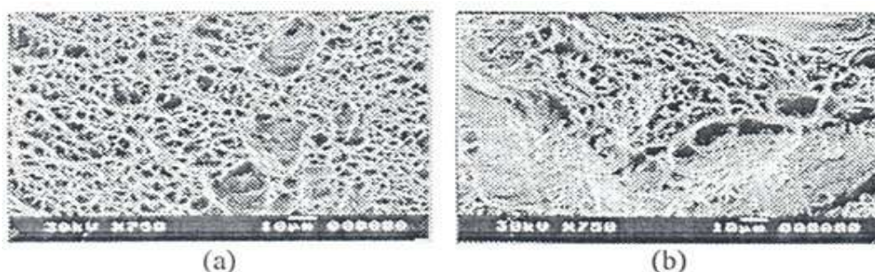
Figure 3: 316 Base metal (a) and 316 weldment (b) tested under controlled potential
