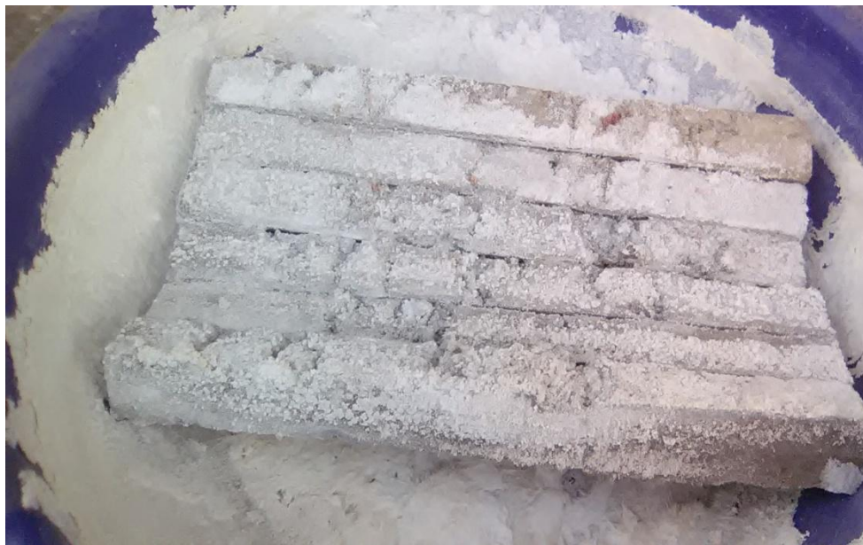
Figure 3: Mortar Bars After Immersion in Sodium Hydroxide (NaOH) solution
