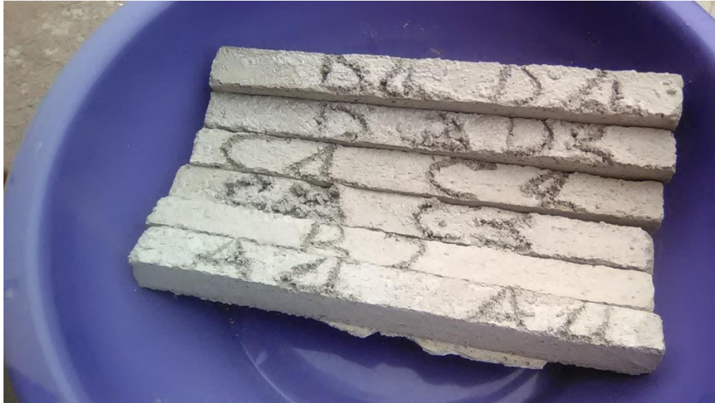
Figure 1: Mortar Bars Before Immersion in Sodium Hydroxide (NaOH) solution
