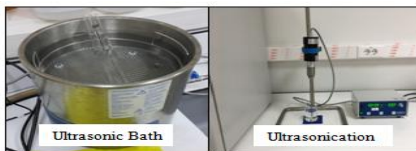
Fig. 1: Digital images of ultrasonic bath and ultrasonication
