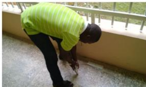
Plate 3: Picture showing Schmidt Hammer Reading of Column and Floor Slab
