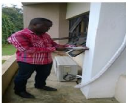
Plate 3: Picture showing Schmidt Hammer Reading of Column and Floor Slab
