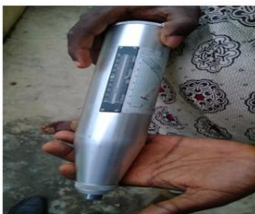
Plate 2: Picture Showing the Schmidt Hammer and Schmidt Hammer Reading of Beam
