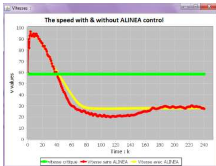
Fig.9: Evolution of speed with & without ALINEA control
