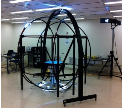
Figure 5: View of the solar simulator of the third type model (HSFL Overvie. 2017 & https://www.hsfl.hawaii.edu/facilities/adcs/ )
