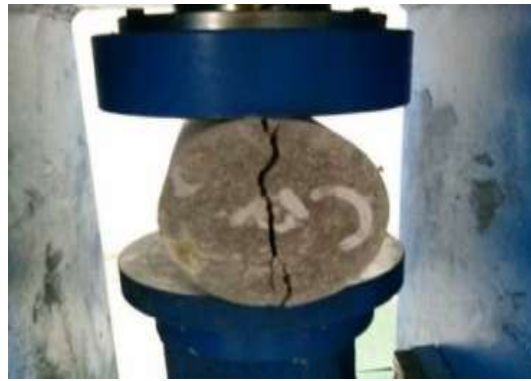
Fig 16: Split tensile testing
