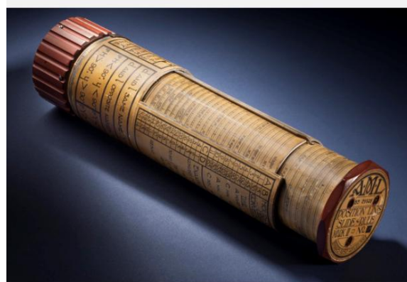
Figure 4. Bygrave position-line slide rule
