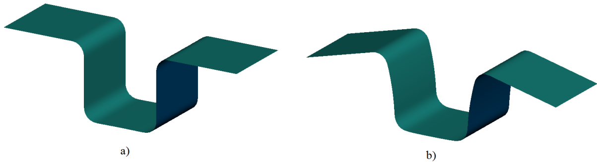
Fig. 3 Formed part before springback calculation (a), formed part after springback calculation (b)
