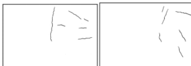
Sketch 5f: Plastic shrinkage cracking 1.0% RP fiber, length 50 mm.
