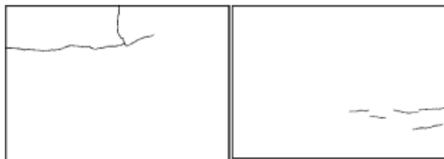
Sketch 5c: Plastic shrinkage cracking 1.0% RP fiber, length 20 mm.
