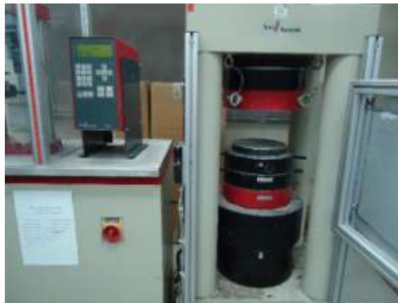
Fig. 4: Compressive strength testing machine.
