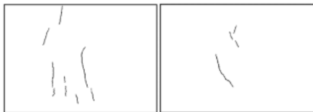
Sketch 5d: Plastic shrinkage cracking 1.50% RP fiber, length 20 mm.
