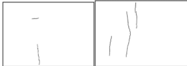
Sketch 5b: Plastic shrinkage cracking 0.50% RP fiber, length 20 mm.
