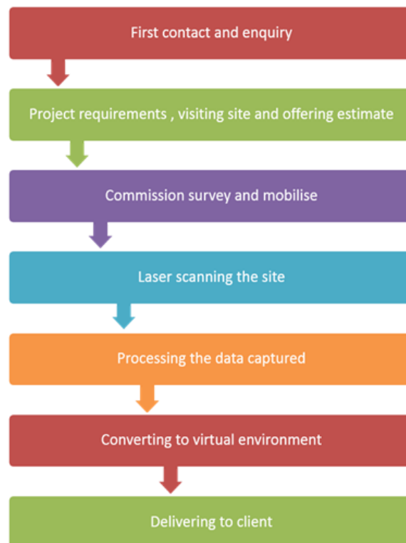
Figure 2: The typical laser scanning survey method.
