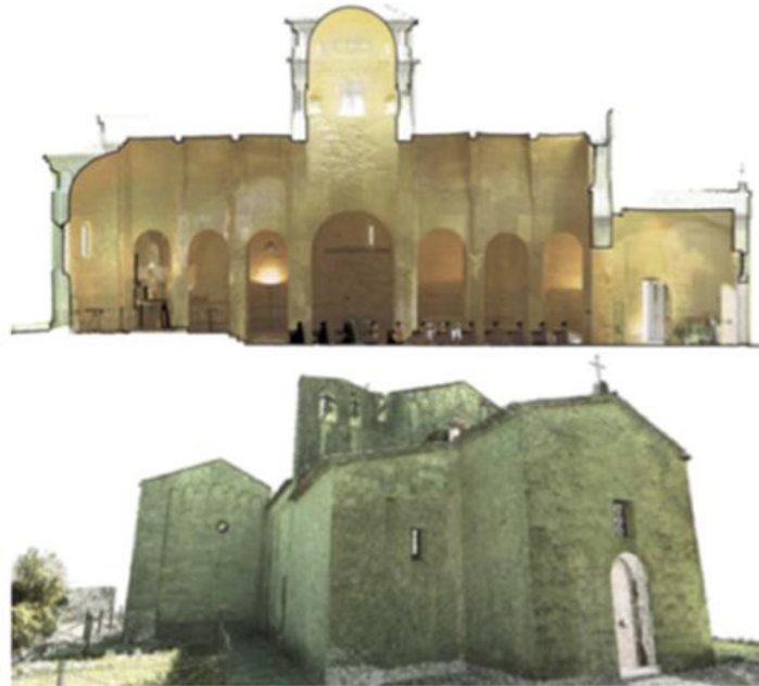
Figure 5: TLS survey of Church Santa Maria at Porto-Novo. Point cloud mapped with the RGB value of camera acquisition done by Quattrini et al. (2015).
