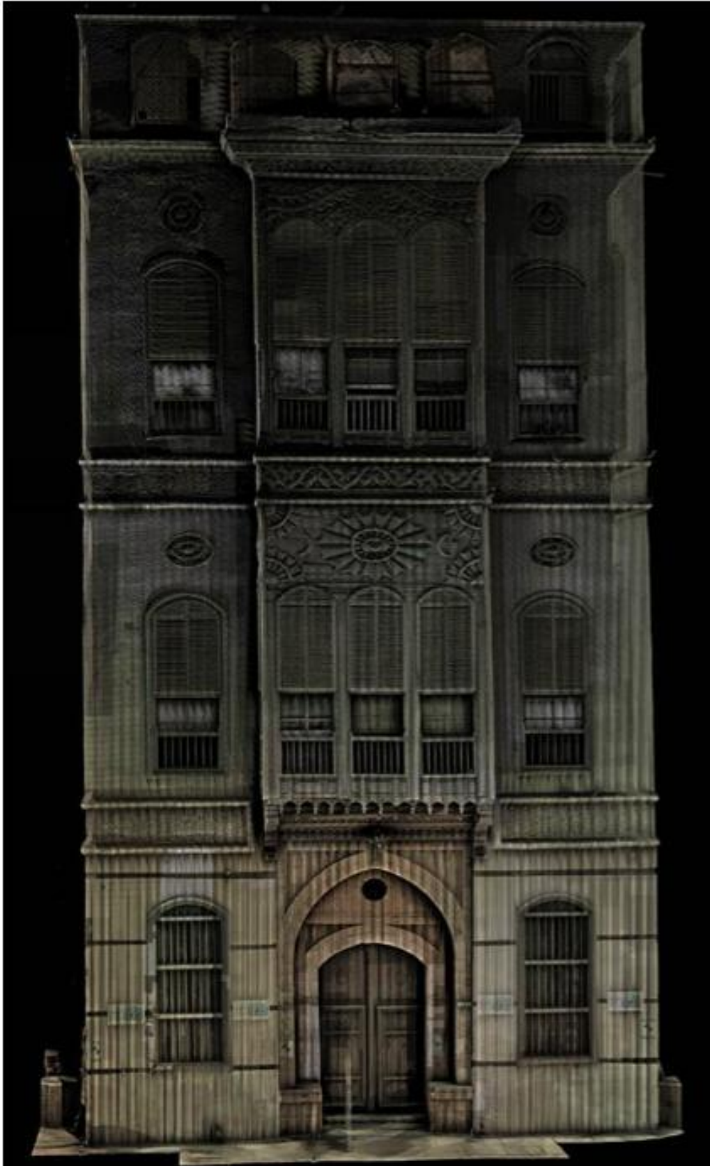
Figure 27: The laser scanning of the main Roshan in Nasif House (the colour is from the scanner).
