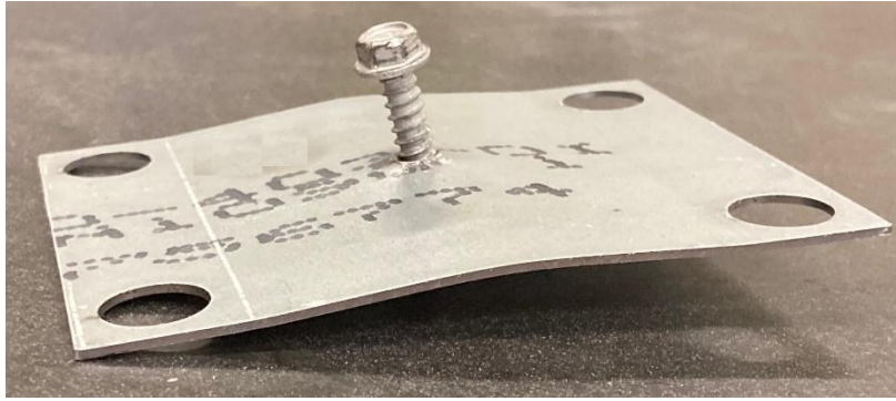
Figure 15. Deformed Sample Due to Maximum Pull-out Force
