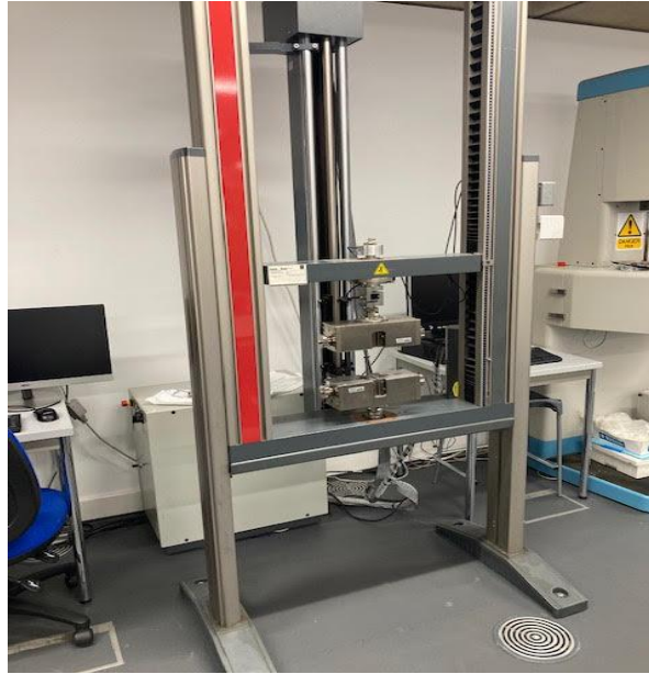
Figure 14. Zwick Z010 Tensile Test Machine with Capacity up to 10 Kn
