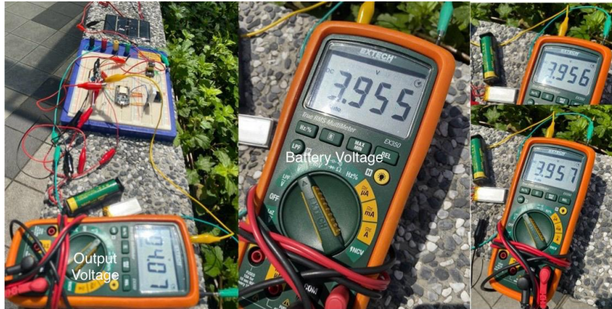
Figure 44: Outdoor Testing (Day mode) and battery voltage
