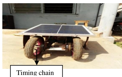
Figure 9: Rear View of the Mower Showing the Timing Chain
