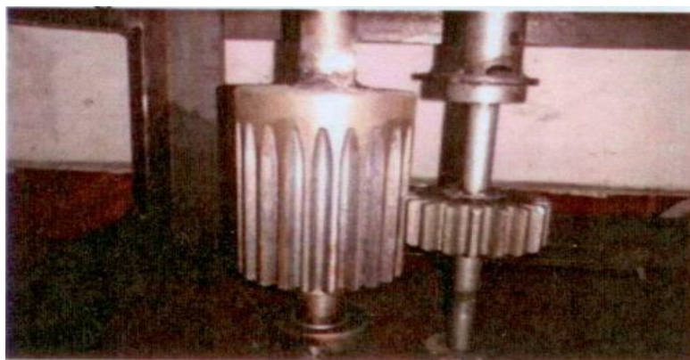
Figure 2: Gear mount of different face width at the cutting deck (Satwik, et al., 2015)
