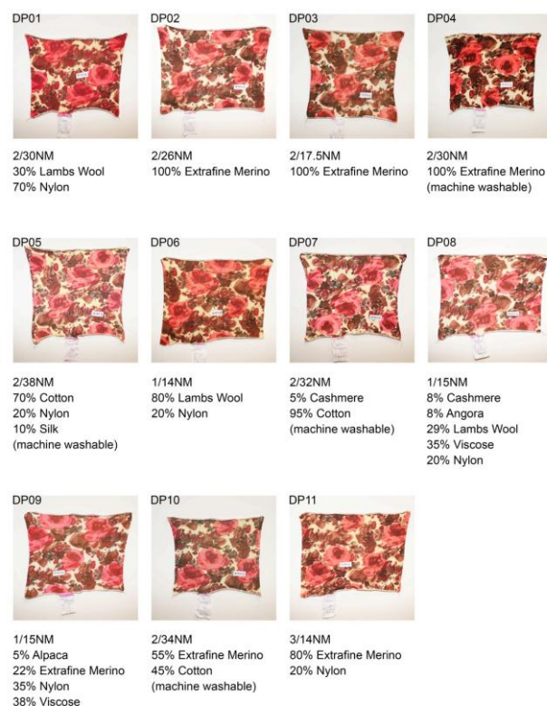
Fig. 4. Color performance and printing accuracy of printed samples with different fiber contents provided by UPW[6]
