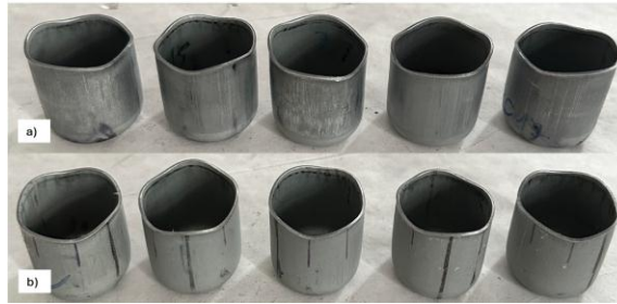
Fig. 3 Cups from material C drawn from a blank diameter of 66 mm, a) without the use of lubricant, b) with the use of lubricant
