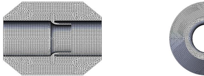
(a) Mesh of Key Components Face-to-face Graph (b) Mesh of Key Components Left View Figure 4 Mesh of Standard Nozzle Core
