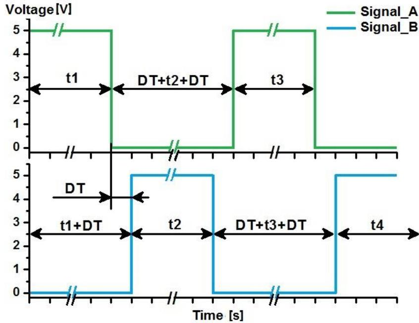
Fig. 2. Gating signals for a single-phase half-bridge inverter.
