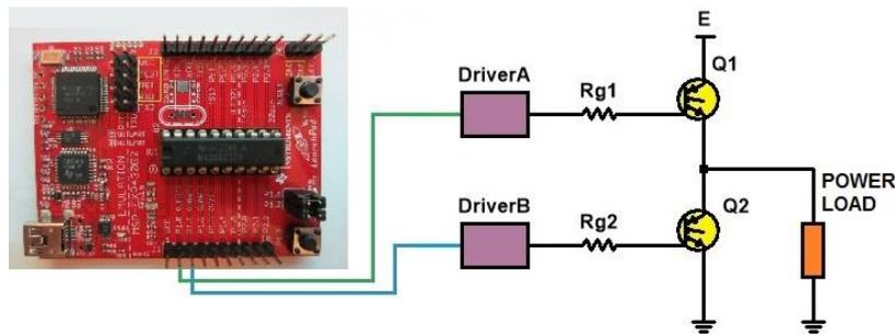
Fig. 3. Schematic diagram for implementation setup.
