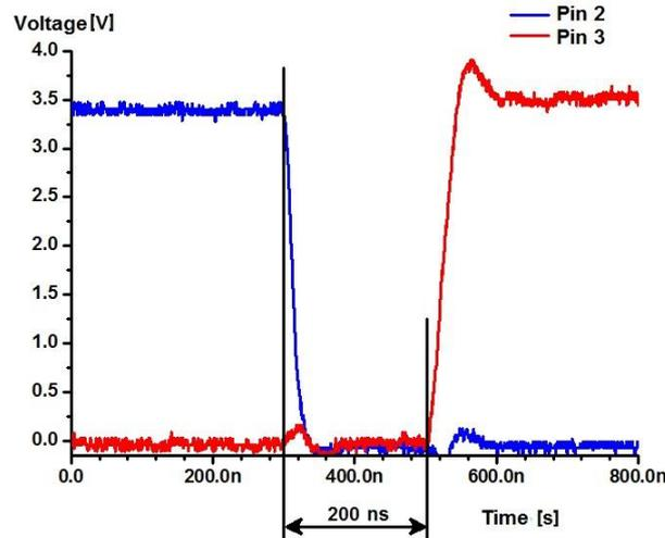
Fig. 7. Dead time obtained from the MSP430G2353 used for gating signals generator for a single-phase inverter controlled by analog input.
