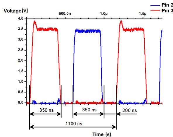
Fig. 4. Obtained signals from implementing assembler code example1 in MSP430G2353 microcontroller.
