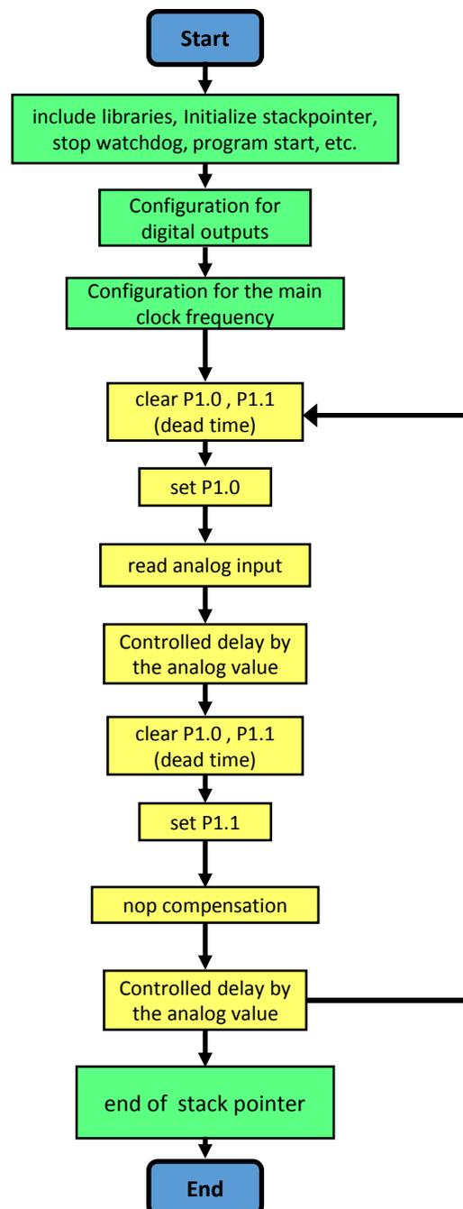
Fig. 5. Flowchart for gating signals controlled by analog input.
