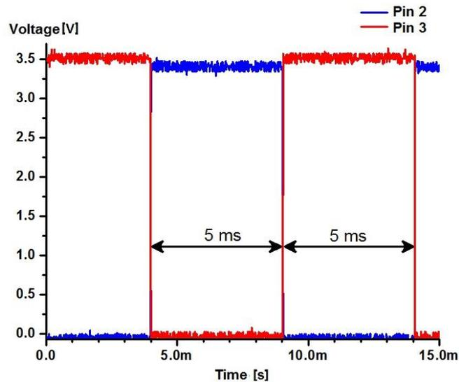
Fig. 6. Generated signals from the implementation of the flowchart of Fig. 5 using the MSP430G2353 controlled by a simple analog input.
