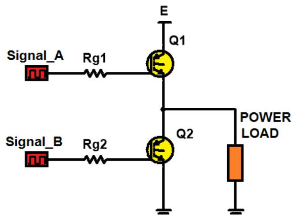
Fig. 1. Single-Phase Half-Bridge Inverter.
