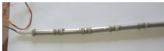
Plate 1. Picture of the Soil Moisture Probe Profile at 5 cm Interval
