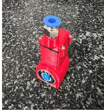
Figure 28 Completed Assembly of Pneumatic Engine
