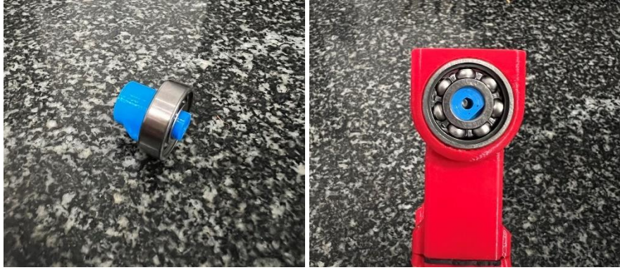
Figure 22 Crankshaft fitted into Ball Bearing then into Crankcase.
