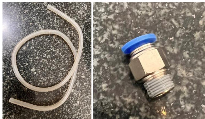
Figure 41 Rubber Hose from an Old Fish Tank Air Pump and Pneumatic Fitting
