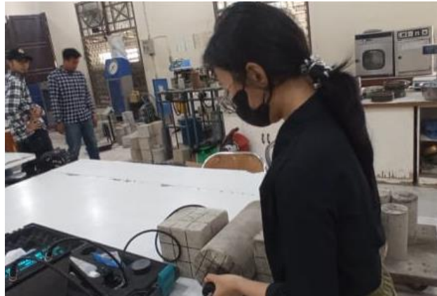
Figure 5. Testing the ultrasonic pulse velocity test method
