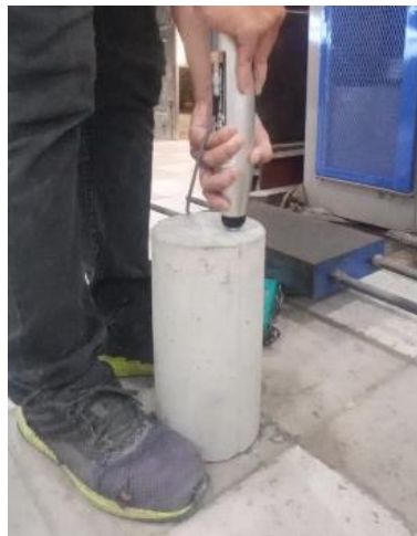
Figure 6. Testing the hammer test method
