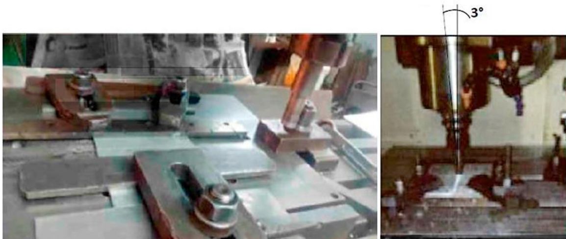
Figure 1. Experimental scheme of FSW welding process.
