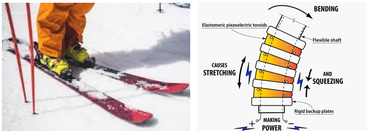
Figure 1-8: Piezoelectrics in snow skis
