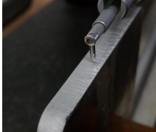
Fig. 7 Measurement with contact roughness meter Mitutoyo SJ 400 sample A 304
