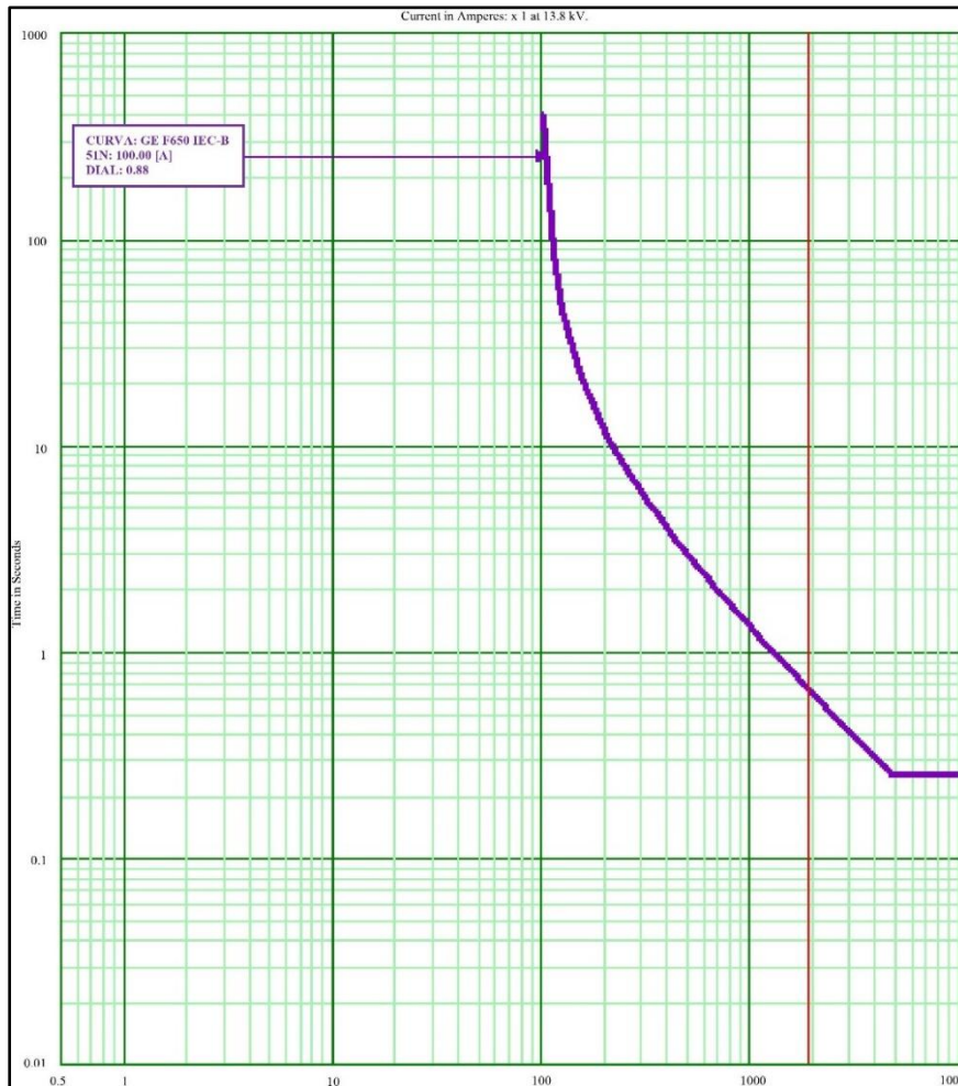
Figure 7: Result of the simulation of the operating time curve of the head switch of Avenida Colon.
