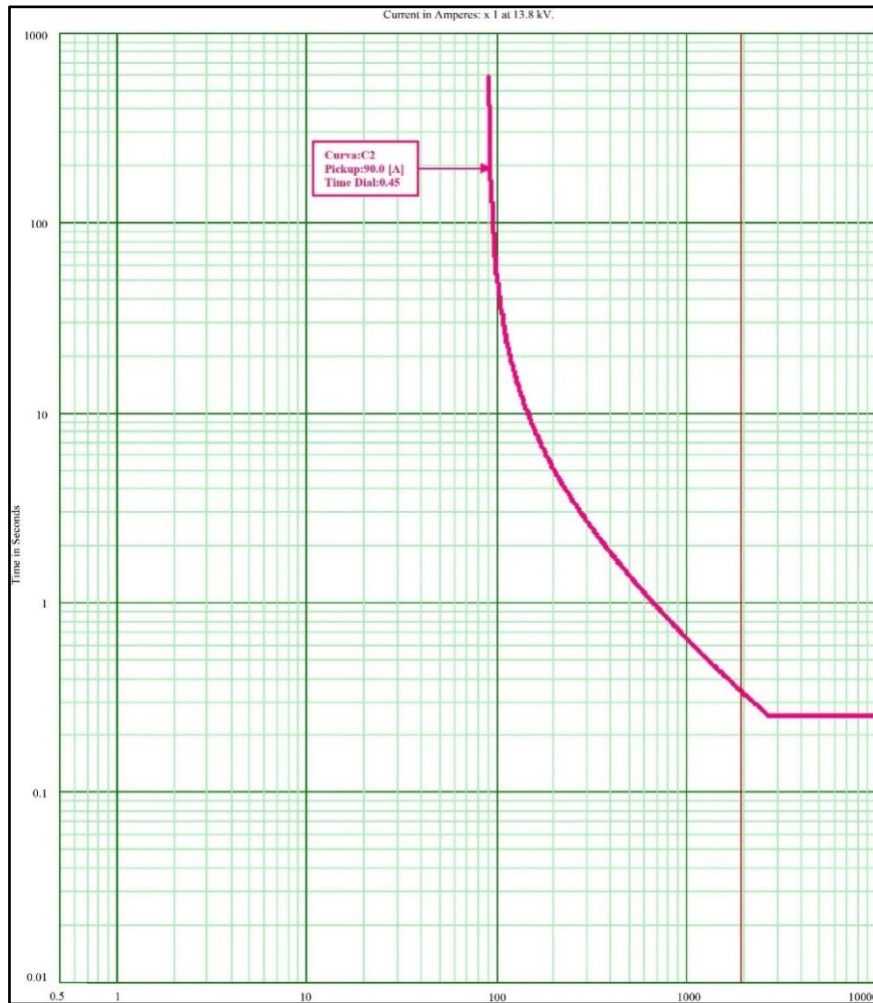
Figure 6: Result of the simulation of the curve of the mid-span recloser of Victor Hugo Vicuña Street.
