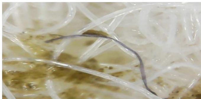
Figure 2: TSS on the felt filter after filtration of the effluent (1600 x magnification)
