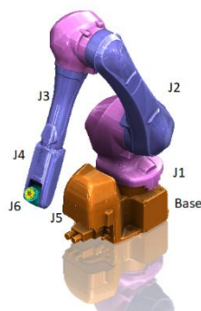
Figure 1: Base and joints
