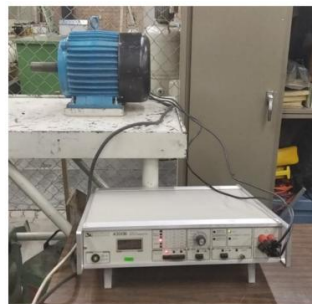
Fig. 15. Physical connection for ohmic resistance measurement
