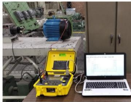
Fig. 16. Physical connection of insulation resistance test
