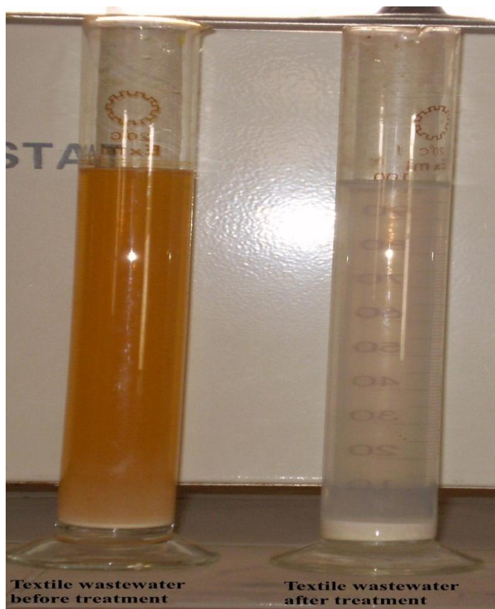
Fig 10. Real textile wastewater before and after photocatalytic irradiation.
