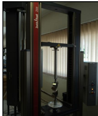
Fig.5 Zwick Roell testing machine (10 KN)
