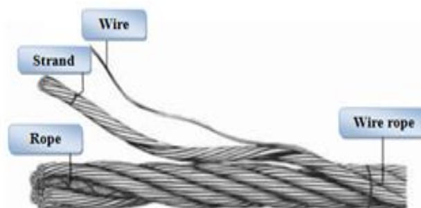
Fig.1 Basic components of a typical wire rope
