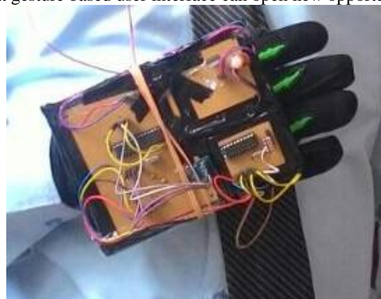
Fig. 7 Gesture Circuit Mounted on Hand Glove
