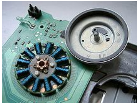
Fig.2. Brushless DC electric motor with floppy disk drive
