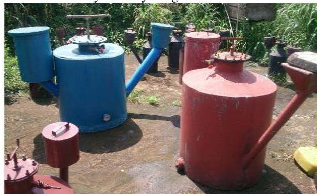
Figure 1: FRP and Metal Digesters
