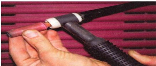
Figure 13 - Install the nozzle (cup) to the torch body.
