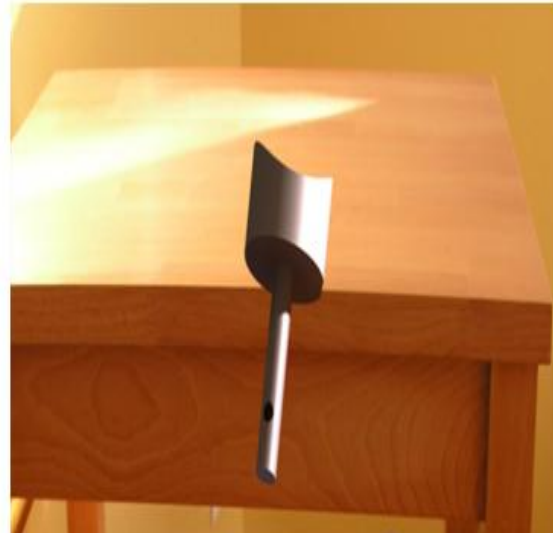
Figure 2 Catia model of piston inside the thermostatic valve
