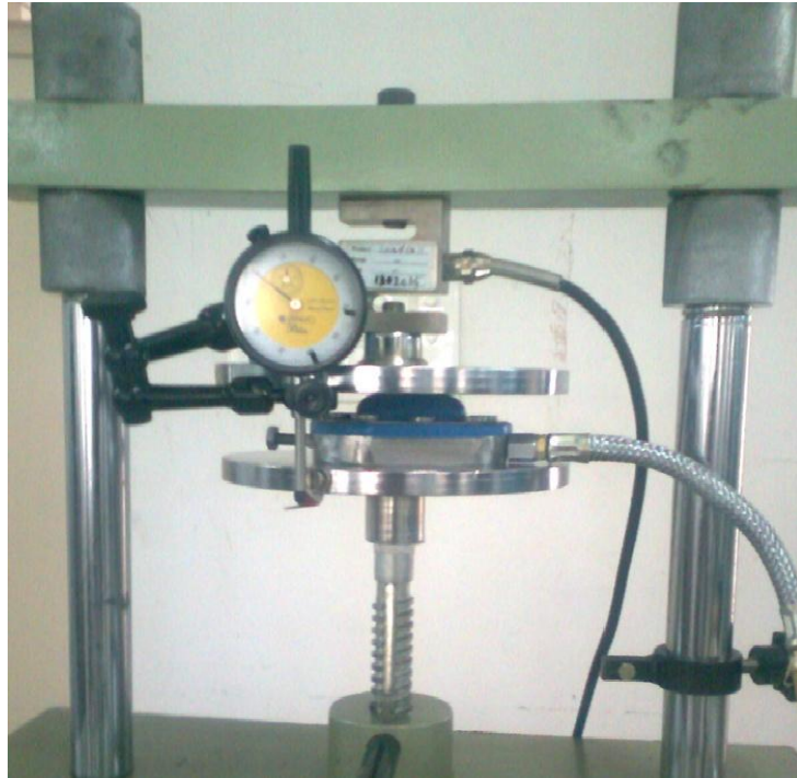
Figure. 3 Finger compression test rig
