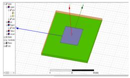
3) Rectangular Patch Antenna with Cylindrical E B G on Roger Substrate
