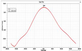
4) Radiation Pattern of L – Slotted Rectangular patch antenna using EBG = 6.658 dB
