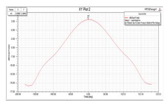
2) Simulated Gain Plot for Rectangular Patch Antenna without E B G on Roger Substrate = 5.6 dB
