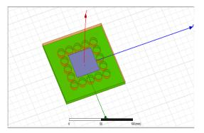
4) L – Slotted rectangular patch antenna with Cylindrical EBG
