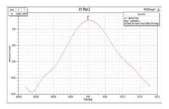
3) Simulated Gain Plot for Rectangular Patch Antenna with Cylindrical EBG on Roger Substrate = 6 dB
