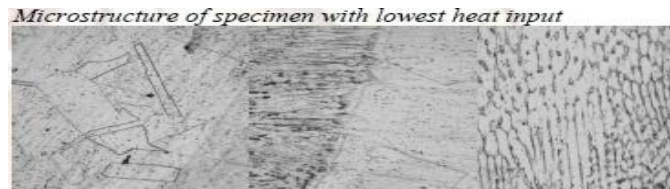
: Microstructure of base metal with HAZ and Weld zone
