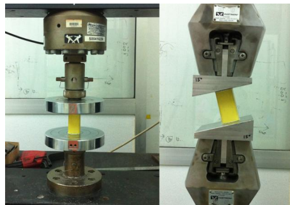
Figure 3: Setup of quasi-static compression test for axially loading (left) and oblique loading (right) with INSTRON 3382 machine.
